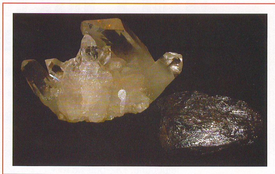
Figure 1. The transformation of quartz to silicon metal is the first step in making silicone compounds. Quartz is on the upper left and silicon on the lower right. (Photo by Thomas O'Lenick, copyright 2005, used by permission)
